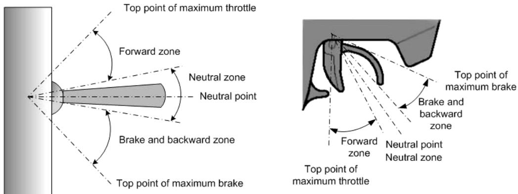
At any time when the throttle is located in neutral zone (except in the throttle calibration or parameters program process), hold the "SET" key for over 3 seconds, the red LED and yellow LED will flash at the same time, which means each programmable item has been reset to its default value.
