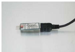
14. With the ESC connected to the **Cirtix ESC PC-USB adaptor**, the Speed passion Software Connection status icons should now both be GREEN.
